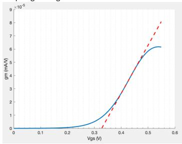
Linear fit line intersects x-axis at Vgs=0.328V
