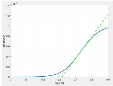
Linear fit line intersects x-axis at Vgs=0.317V So Vgs=Vth = 0.317V
