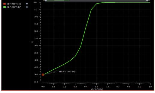
The worst-case capacitance is when the pn juntions (D-B and S-B) are unbiased. The value of worst-case capacitance Cdb and Csb is 50.1aF as shown from the above graph.
