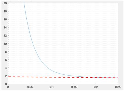
From the above graph and fit line,  $\lambda = 1.76 \text{ V}^{-1}$   $\lambda \cdot L = 1.76 \text{ V}^{-1} * 50 \text{nm} = 88 \text{ nm/V}$
