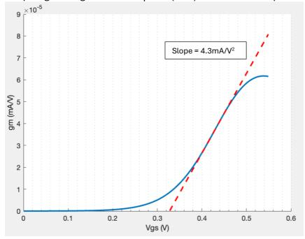
From the above graph, slope of linear fit line =  $4.3 \text{ mA/V}^2$   $\mu\text{Cox}$  (W/L) = 0.0043 Since W/L = 12  $\mu\text{Cox}$  = 0.0043/12 =  $358.33 \text{ uA/V}^2$
