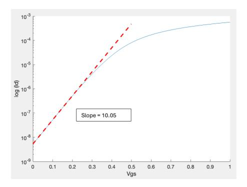
From the above graph, Slope of fit line =  $10.05 = 1/(2.3*n*V_T)$
